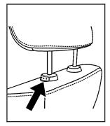
Press the button on the side of the head restraint to lower it.
